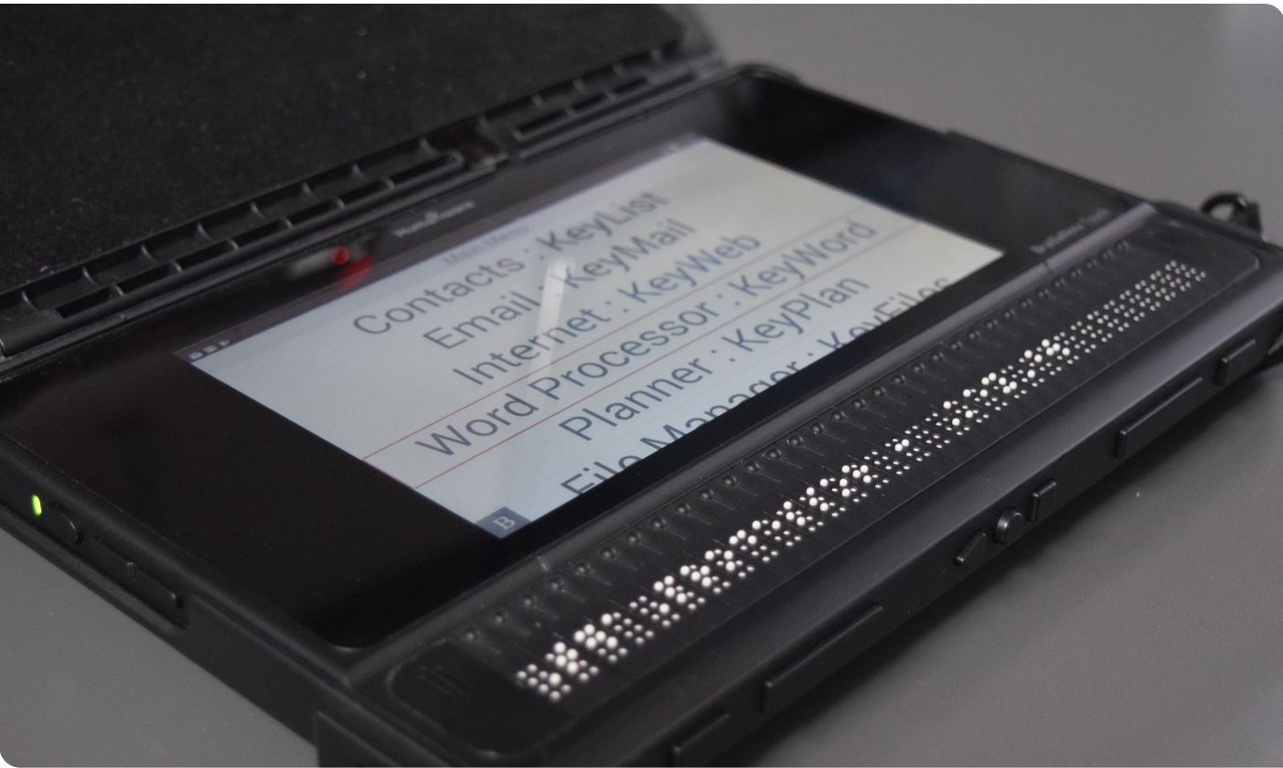
Braille readers read documents, emails and webpage text using the refreshable braille display at the bottom of BrailleNote devices like this.
